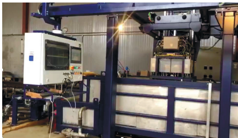
Fig. 9. General appearance of the NORDINSCAN-RAIL-S (Nordinkraft) installation of ultrasonic quality control of rail surface in the line of acceptance testing of rails at a metallurgical enterprise.
